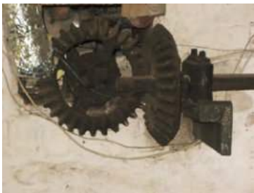
Right angle bevel gearing that once worked the waterwheel sluice from inside the old sawmill
