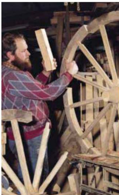
Wheelwright hammering felloes onto spokes, Devon
